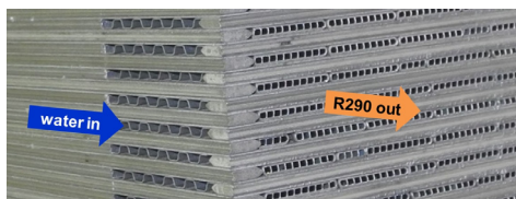
Prototype Aluminium condenser with counter-current flow of refrigerant and water
